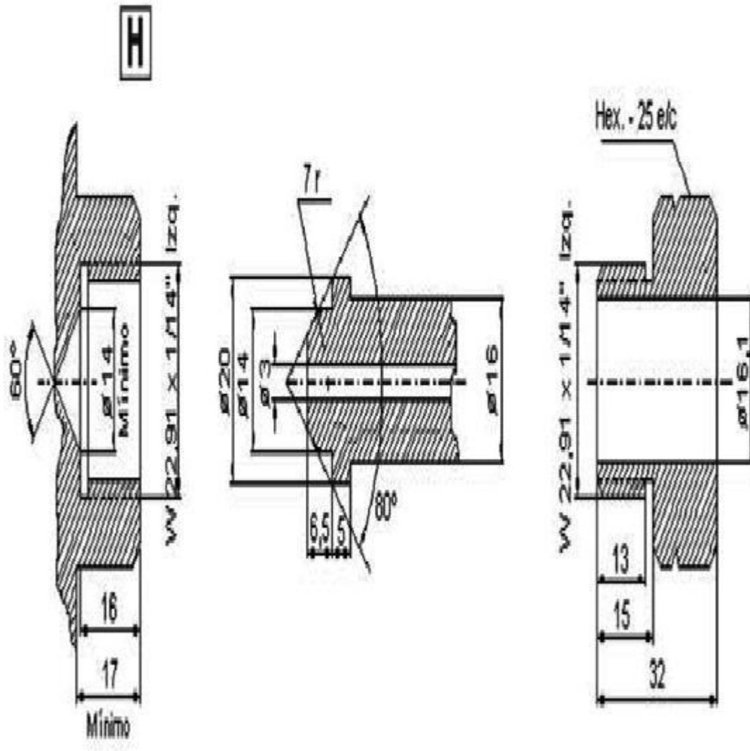
ACOPLAMIENTO W 22,91 - 14 Hilos/Pulgada (IZQUIERDAS).
