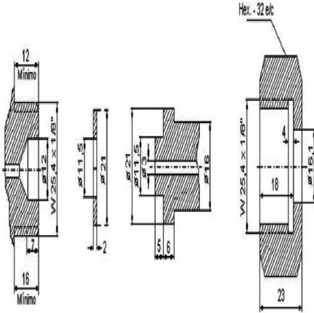
ACOPLAMIENTO W 25,4 - 8 Hilos/Pulgada (DERECHA).
